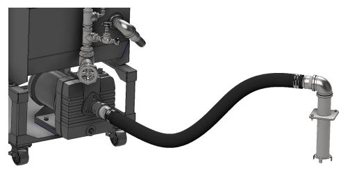
2) REQUIRED, using provided worm drive clamps (2ea) connect 1-1/2" overflow braided hose (transparent) to 1-1/2" barbed nipple located on back of ATMS unit. (Loosely install worm drive clamps on hose prior to sliding hose on barbed nipple for ease of installation.)
