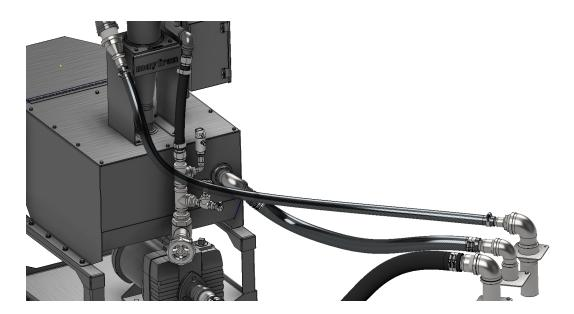
4) OPTIONAL, using provided worm drive clamp (lea) connect 1/2" tank agitator braided hose (transparent) to 1/2" barbed nipple located on 1/2" valve on ATMS unit. (Loosely install worm drive clamps on hose prior to sliding hose on barbed nipple for ease of installation.)
