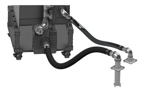
3) REQUIRED, using provided worm drive clamp (1ea) connect 1" return truck hose (black) to 1" barbed nipple located on AT-Cleaner on ATMS unit. (Loosely install worm drive clamps on hose prior to sliding hose on barbed nipple for ease of installation.)
