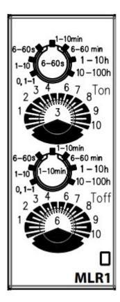
The (2) upper-most dials control the cycle-on time  $(T_{on})$  while the (2) lowest dials control the time between cycles  $(T_{off})$ . To adjust the timer, select the range that includes your desired setting in the upper dial, then select the k-factor on the lower dial. The k-factor represents the percentage (in tenths) of the upper-limit of the range.
