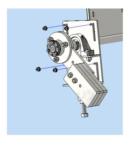
2) After the (8) nuts are loosened, loosen the Take-up nut, and adjust the take-up. (See below)
